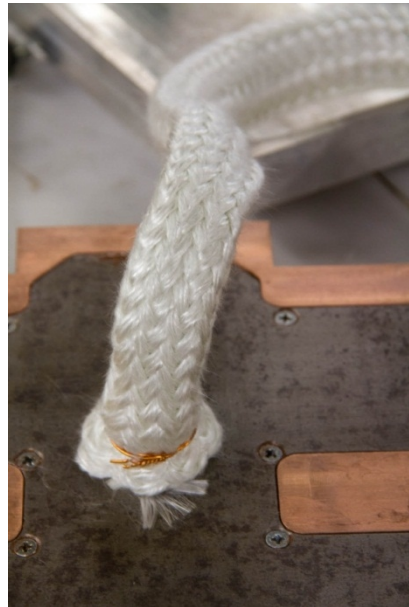
Figure 31 - Protection of the thermocouple wires in the test mold.
