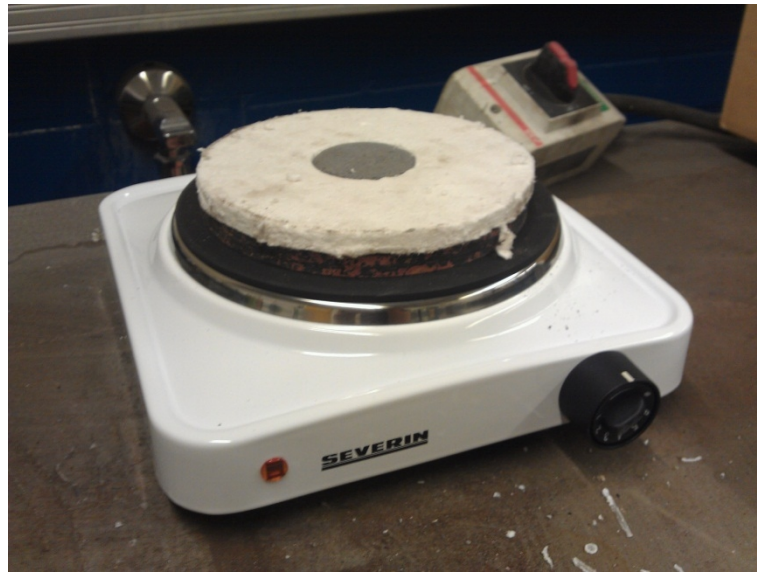
Figure 24 - The hot-plate with the insulation and core material sample placed inside the insulation ring in the thermal conductivity studies of core sands.
