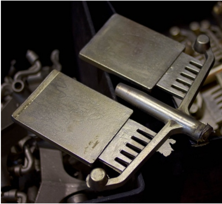
Figure 35 - Test castings produced in the casting experiments
