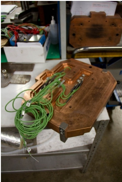
Figure 30 - Instrumentation of the mold
