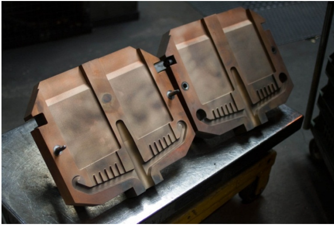
Figure 29 - The sample cavities of the instrumented test molds.
